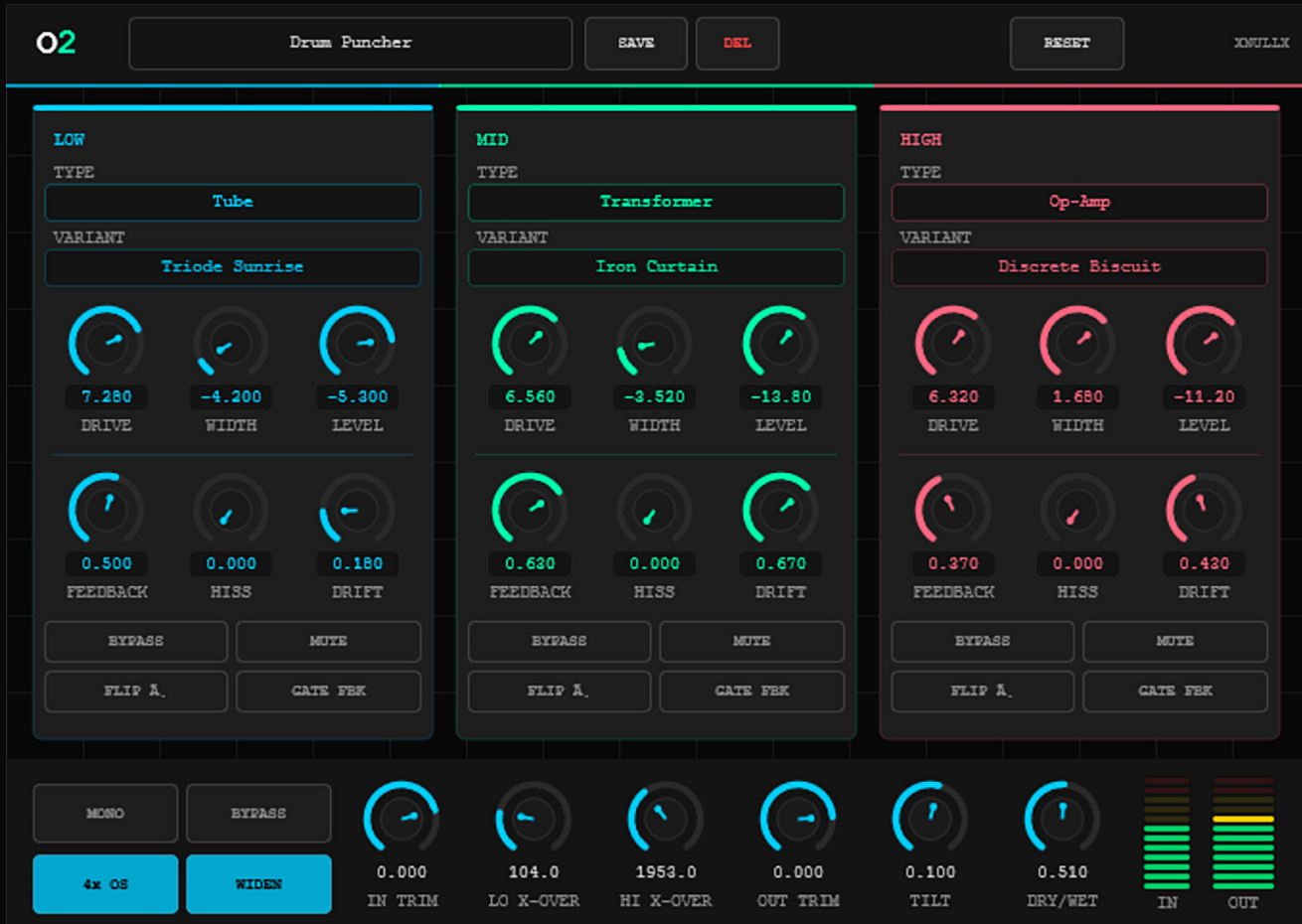
The O2 interface: top bar, three band strips (Low / Mid / High), and the global bottom bar (In Trim, crossovers, Out Trim, Tilt, Dry/Wet).
