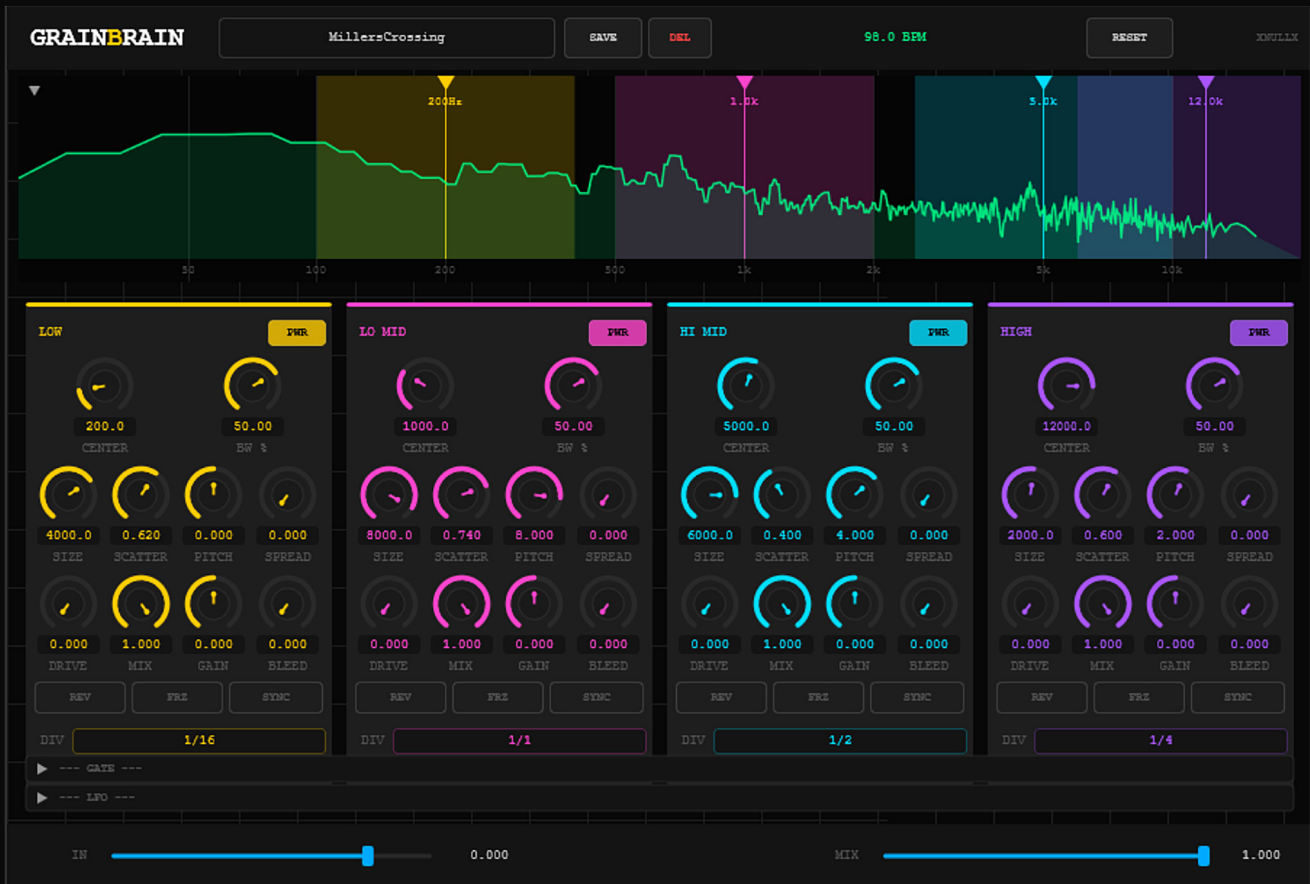
GrainBrain at its most compact: the frequency display condensed and the GATE and LFO sections collapsed. The window resizes to fit, leaving just the band filter and grain controls.
